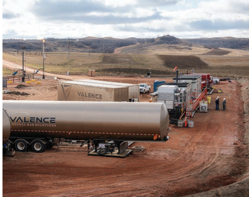
Left: A Valence microplant moves from site to site to capture otherwise flared gas. Right: Valence trucks and trailers move compressed natural gas around the basin.
