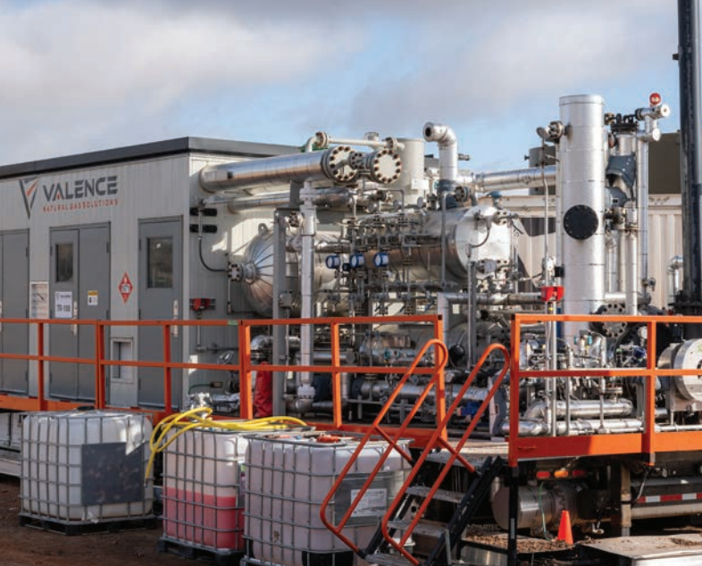
Left: A Valence microplant moves from site to site to capture otherwise flared gas. Right: Valence trucks and trailers move compressed natural gas around the basin.
