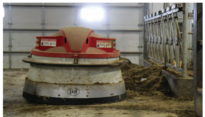
This 4-foot wide robot looks like a household Roomba vacuum, but instead of vacuuming, it pushes the feed closer to the cows so they are able to eat.
